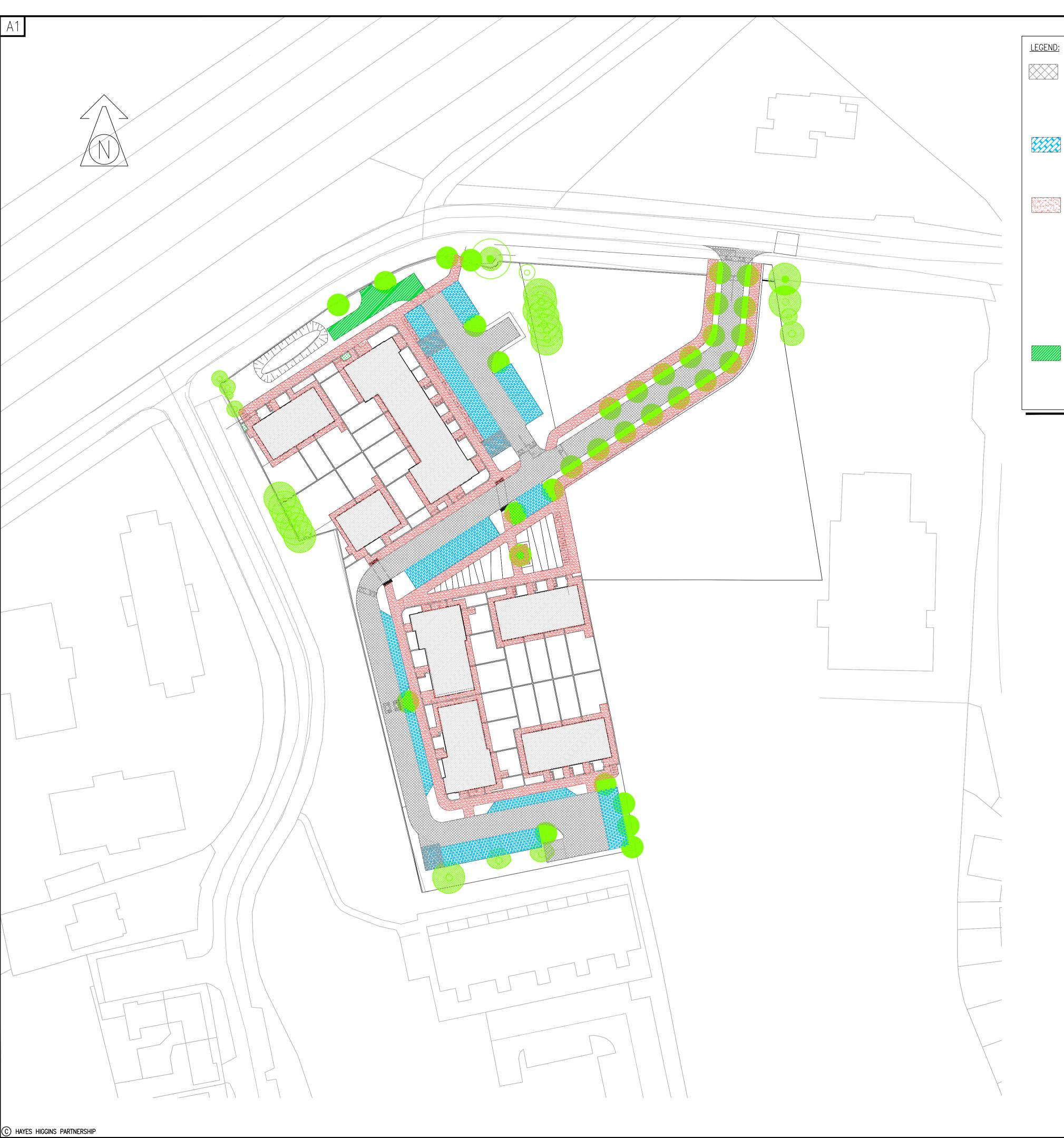
PROPOSED ACCESS ROAD/TURNING AREA 45MM OF SMA 14 SURF PMB 65/105-60 CLAUSE 942 ON 80MM OF ACBC (28) BASE COURSE ON 150MM ANNEX E T1 STONE ON
